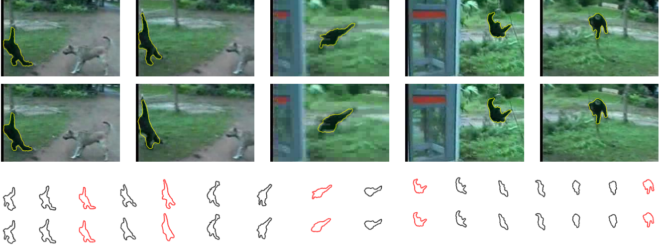
Figure 4: Video Segmentation Example: We segmented 48 frames of the "monkey" sequence from the SegTrack database of Tsai et al. [28]. First row: Five frames with the segmentations obtained with the method of Papazoglou and Ferrari [18]. Second row: The same frames with segmentations regularized with our algorithm. Third row: Shape signal consisting of the original segmentations, where only every third shape is displayed for better visibility. The shapes corresponding to the frames in the upper two rows are highlighted in red. Fourth row: Regularized shape signal with the same shapes highlighted.
