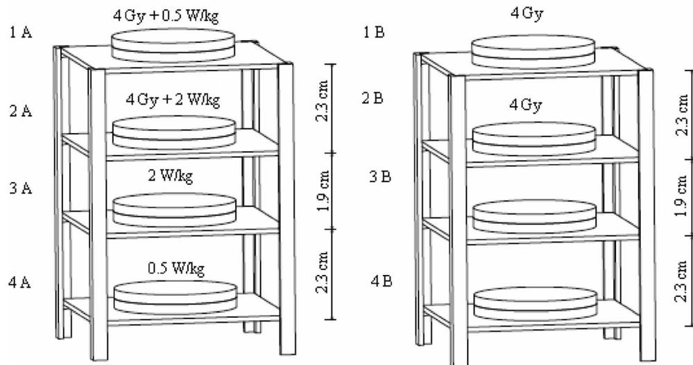
**FIG. 1.** Panel A: Arrangement of the petri dishes and plastic stand in the waveguide. Panel B: Sketch of the configuration adopted for the positioning of the biological samples inside the waveguide. The samples denoted as B are placed in the second waveguide in the absence of the RF signal.
