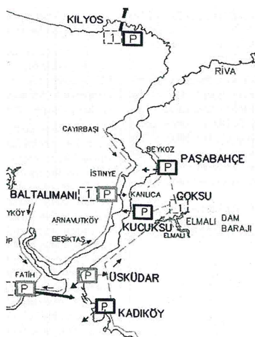
FIGURE 2 - ISKI wastewater discharges along the Strait coastline (Squares with P show the discharge points) [33].
