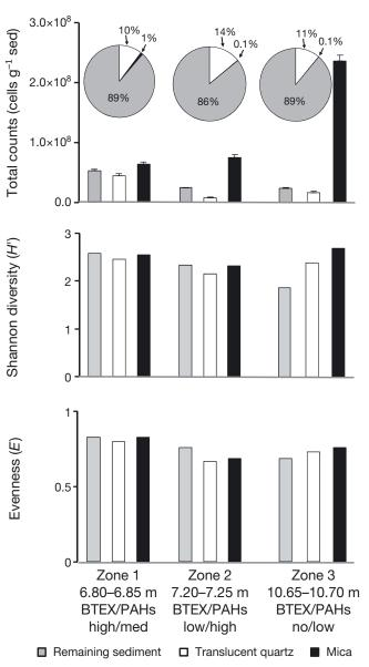
Fig. 2. Total cell counts, Shannon diversity (H'), and evenness (E) of bacterial communities attached to different sediment (sed) mineral fractions from 3 zones of varying contamination in a sandy aquifer contaminated with petroleum hydrocarbons. Pie charts refer to the relative abundance of the sediment mineral fractions. BTEX: benzene, toluene, ethylbenzene, and xylenes; PAH: polycyclic aromatic hydrocarbons
