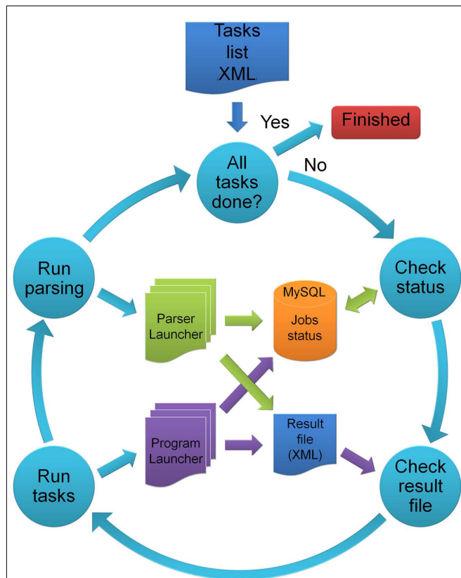
FIGURE 3 | Schematic representation of the master program (MP).
