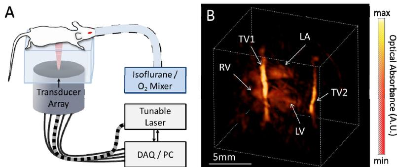
**Figure 1:** Schematic of the experimental setup (A), and representative 3D optoacoustic image of the mouse heart (B). Important structures are identified and annotated in the optoacoustic image: RV, right ventricle; LV, left ventricle; LA, left atrium; and TV1 and TV2, thoracic vessels 1 and 2.
