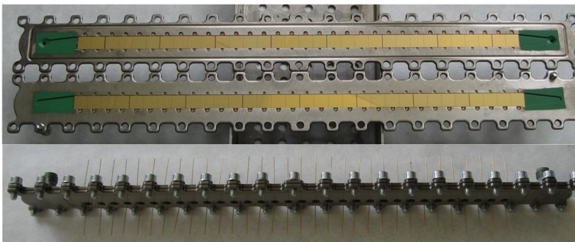
Figure 2. TUM4/Au array - inside of the array and the assembled array
