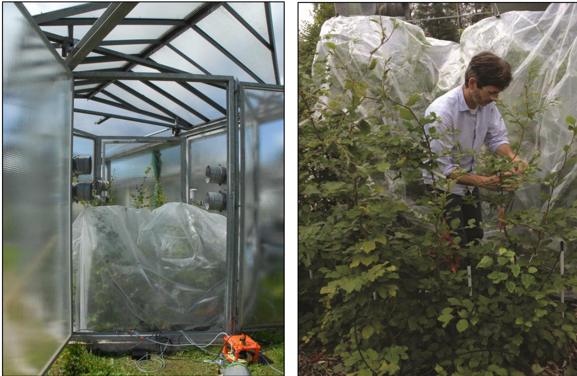
Supplementary Figure 1: Field-based open top chamber/lysimeter with beech model ecosystems during the ^{13}\text{C} pulse labelling. The chambers have a height of 3.5 m and a plantable area of 3 m 2 for each of two lysimeters inside the chamber (only one lysimeter used for the experiments). The beech trees were up to 2.5 m tall at the time of the experiments.
