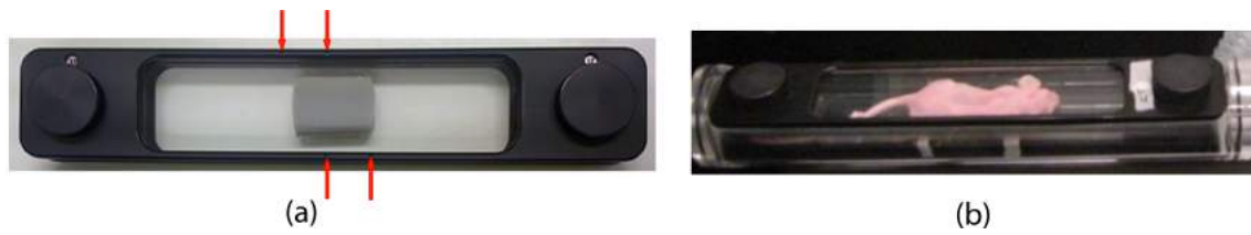
Figure 4.2: FMT imaging cartridge containing (a) a phantom and (b) a mouse. Small holes in the non-transparent margin of the cartridge serve as fiducial markers (arrows).
