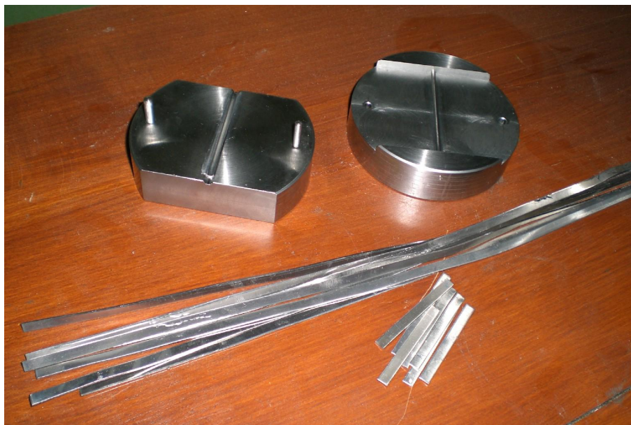
Figure 5. The lead stripes and the pressing form for obtaining the shields
