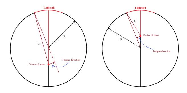
Fig. 8. Scheme of torque directions in case of  $L_c > R$  (left panel) and  $L_c < R$  (right panel).
