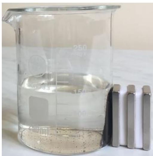
Figure 2. The photograph showing the recovery of MNC from its suspension by application of external magnetic field (neodymium magnets).
