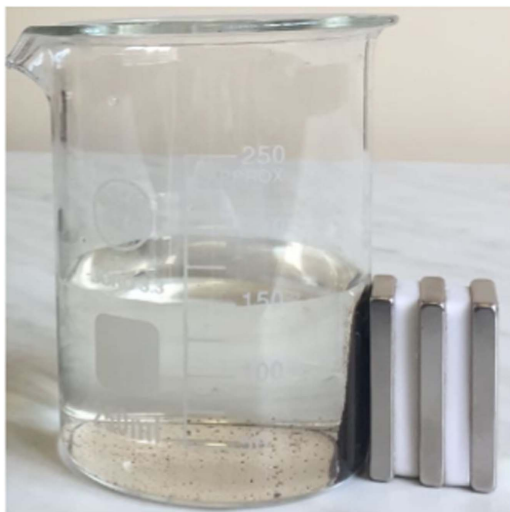
Figure 2. Photograph showing the recovery of MNC from its suspension by application of external magnetic field (neodymium magnets).
