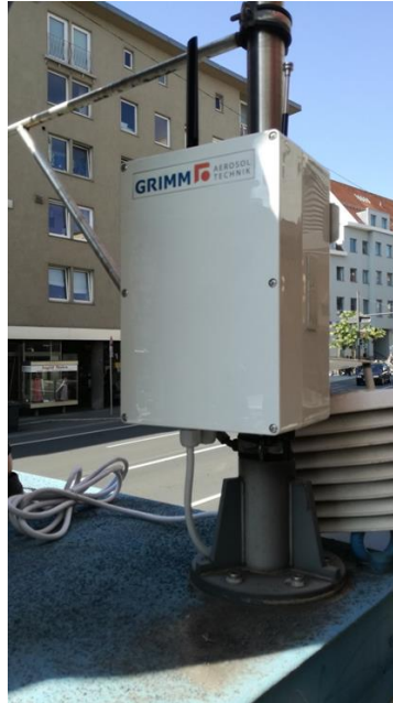
Figure 2. Prototype nephelometer EDM80 Neph called here scout (autonomous, mobile smart dust measurement device that is auto-calibrated to a high-quality reference instrument within an intelligent monitoring network) installed at the state air quality monitoring station Karlstrasse.
