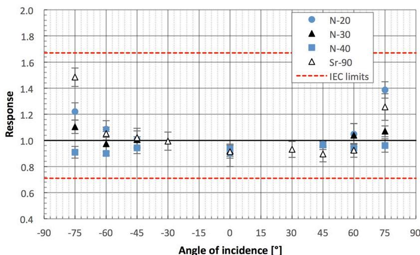
**Figure 14** Response to the lowest photon energies N-20, N-30, N-40 and to 0.8 MeV betas from  $^{90}\text{Sr}/^{90}\text{Y}$ , measured over an angular range of incidence of  $\pm 75^\circ$ . The dashed lines denote the IEC limits.
