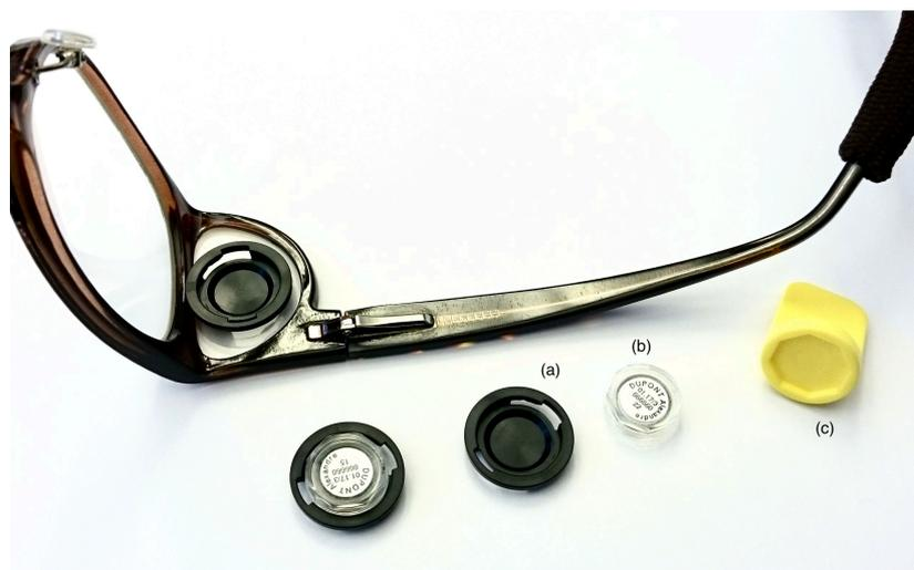
Figure 7 Adhesive adapter (a) with Dosilab TLD ELD (b) and insertion key (c).
