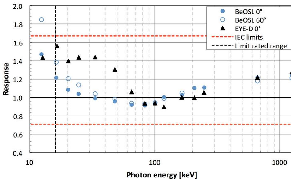
Figure 8 Energy response of the BeOSL ELD for  $0^\circ$  and  $60^\circ$  photon incidence.
