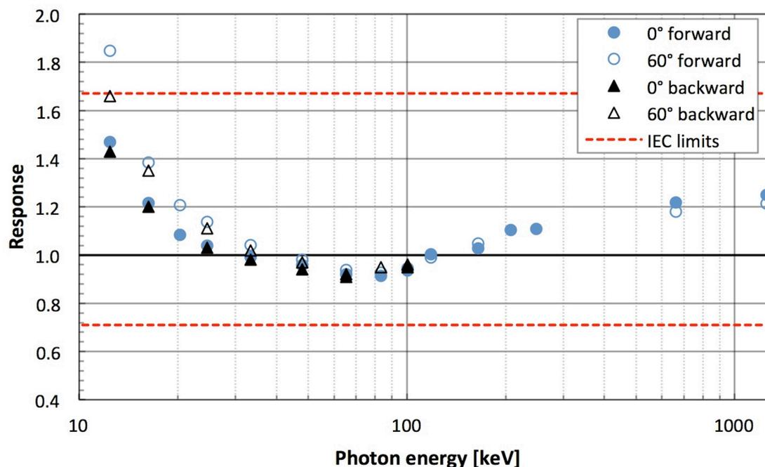
Figure 9 Energy response for backward and forward irradiation: there is no difference in response due to the symmetrical design.
