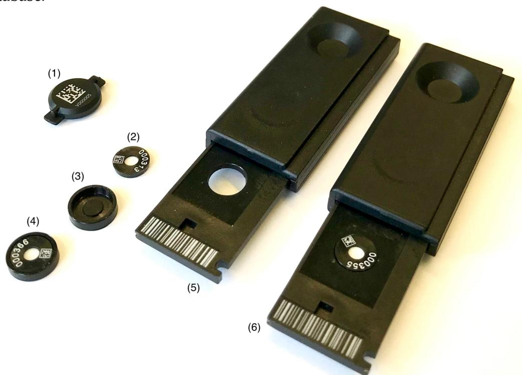
Figure 3 ELD with BeOSL detector element and readout badge: (1) ELD front enclosure, (2) ezClip detector element, (3) detector tray, (4) tray with ezClip inside, (5) readout badge ezCase, (6) ezCase with ezClip inserted.
