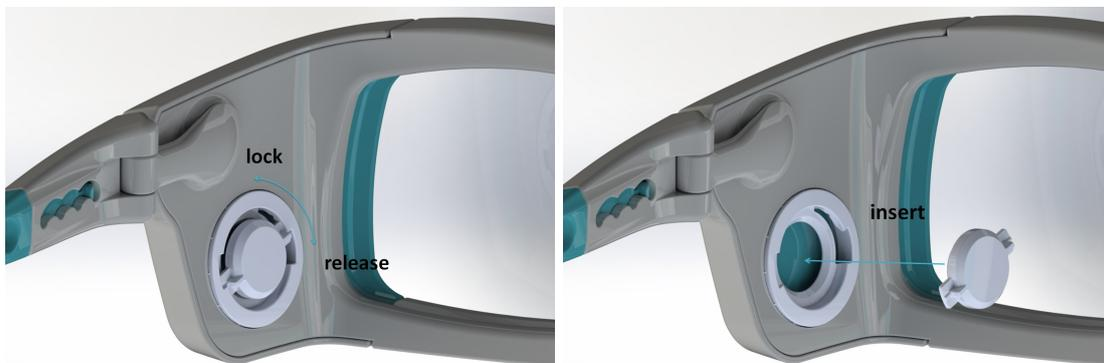
**Figure 2** Bayonet coupling between RP glasses and BeOSL ELD. Left: Open coupling, showing the recesses engaging with the small fins which protrude from the dosimeter housing. Right: Quick and safe locking and releasing of the dosimeter by means of the bayonet mechanism.
