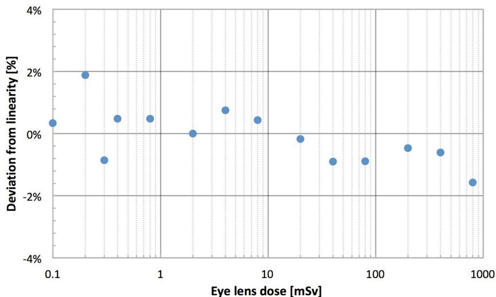
Figure 12: Dose linearity: the ELDs deviate less than 2% from linearity for doses from 0.1 mSv to 1 Sv. IEC limits are -13% to +18%.
