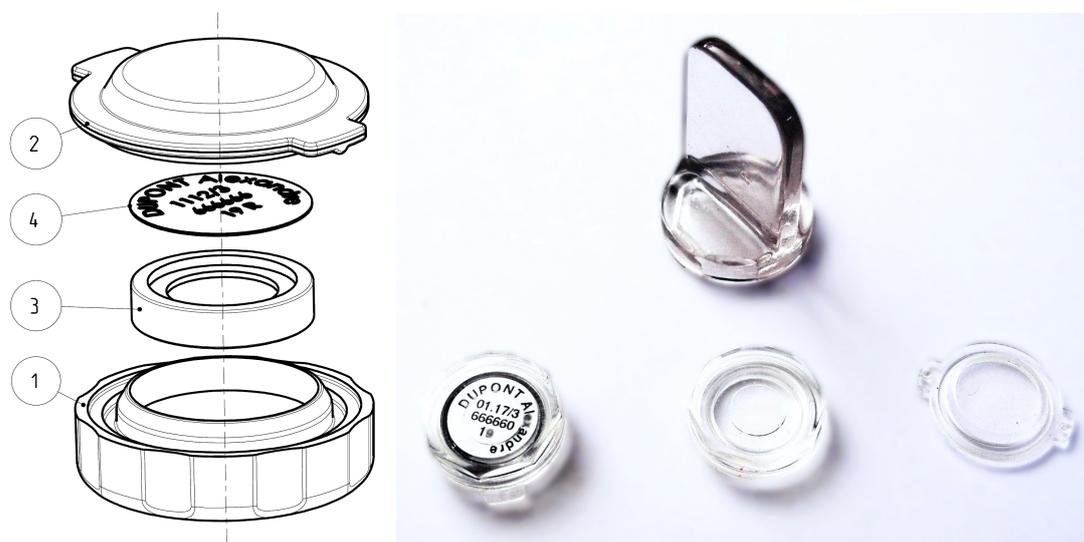
**Figure 5** The schematic assembly of the dosemeter (left) comprises the 3mm front cap (1) where the TL detector (3) is inserted, followed by a label (4) with information like personal name, wear month, detector ID, finally being enclosed and hermetically sealed with the thin back cap (2) through ultrasonic welding. The photograph (right) shows both housing sides and the assembled  $H_p(3)$  dosemeter. A key is supplied for safe and easy manipulation.
