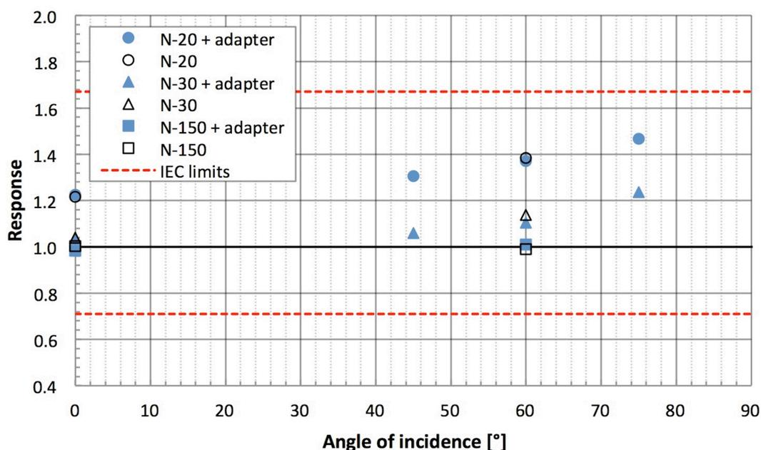
Figure 10 Angular response of dosimeters irradiated in the headband adaptor is the same as without the adaptor.
