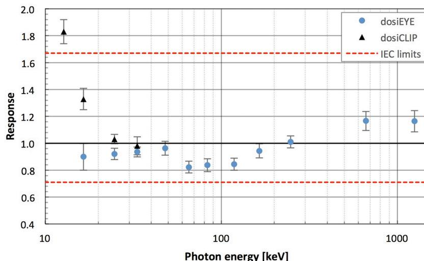
**Figure 13** Energy response of the  $H_p(3)$  dosimeter (dosiEYE, solid circles). For comparison, the response of a  $H_p(0.07)$  dosimeter (dosiCLIP, solid triangles) is also shown. The dashed lines denote the IEC limits.
