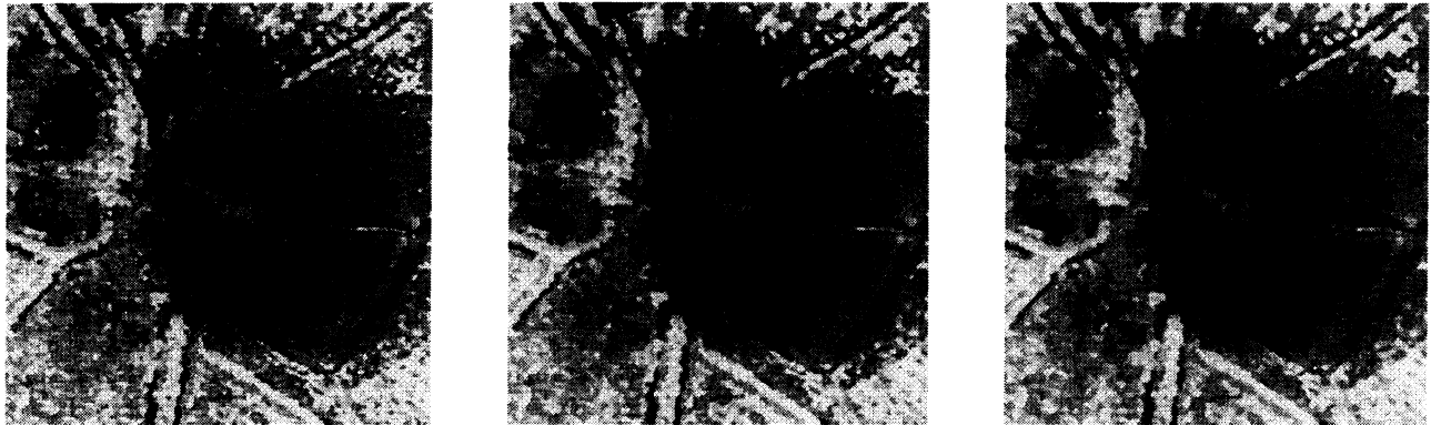
Fig. 11: Iterative improvement of the surface information. The three presented range images (from left to right) show the several results of the improvement steps after the first, second and third iteration. A replacement-tolerance of two depth units is used. During each iteration larger defects will shrink more and more, until they disappear. Each iteration achieves a visible improved homogeneity of the surface and the mean of the amount of changes of the depth information in each iteration decreases in about 50%.
