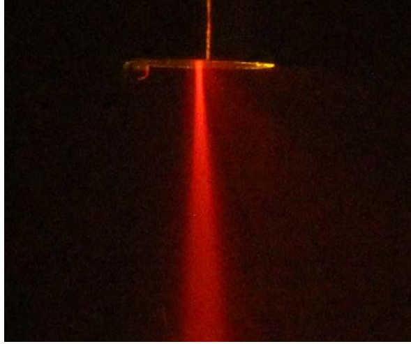
Figure 5.27: A picture of the multimode fiber illumination coming out of a transducer in water.
