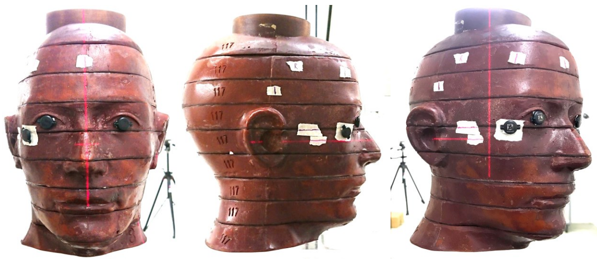
Figure 1 Alderson-Rando head phantom equipped with dosimeters on eyes and temple for baseline irradiations. Laser lines aid in positioning of the phantom in the beam centre and at the distance of 2 m.
