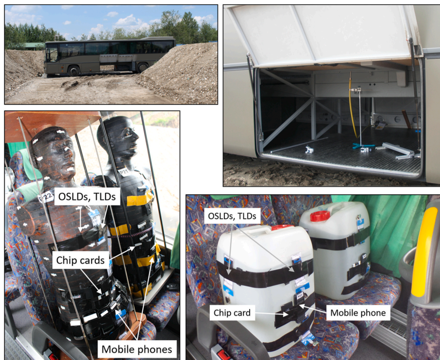
Fig. 1. View of the bus (top left), the end tip of the guide tube of the source in the compartment area (top right), anthropomorphic phantom (bottom left) and water canister (bottom right), equipped with mobile phones, chip cards (wrapped in black bag) and personal dosimeters.
