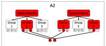
**FIGURE 3** | Illustration of a simple A2 procedure where the positive individuals are uniquely determinable after the first stage. Every individual  $a, b, c, \ldots, i$  gets pooled exactly twice.
