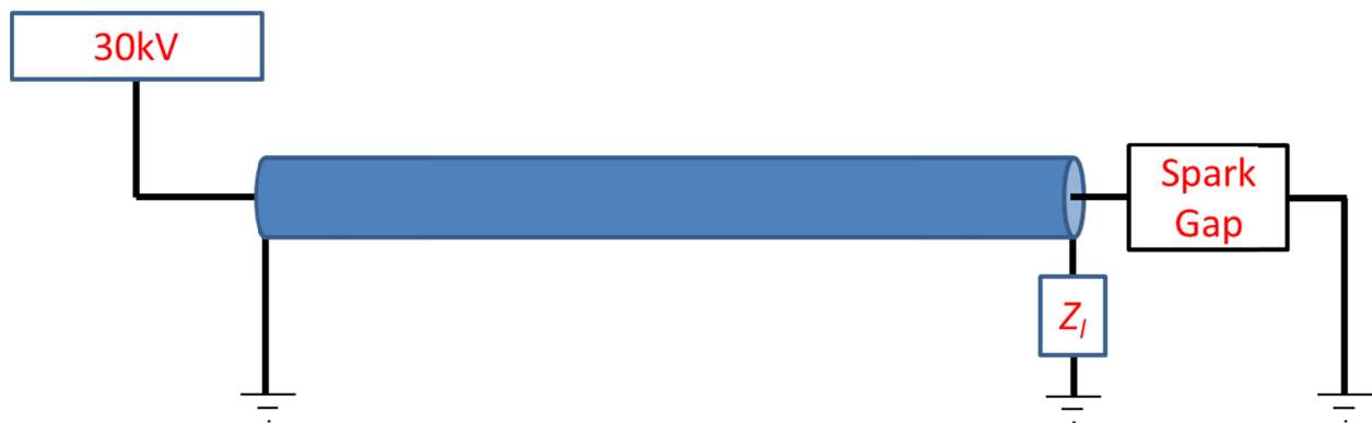
Fig. 2: the transmission line based impulse generator.
