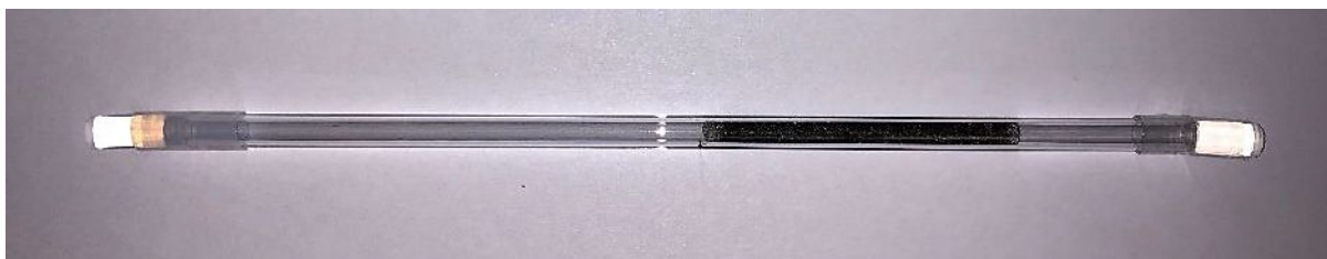
Figure S1: Optimized graphene wool (GW) sampler assembly.
