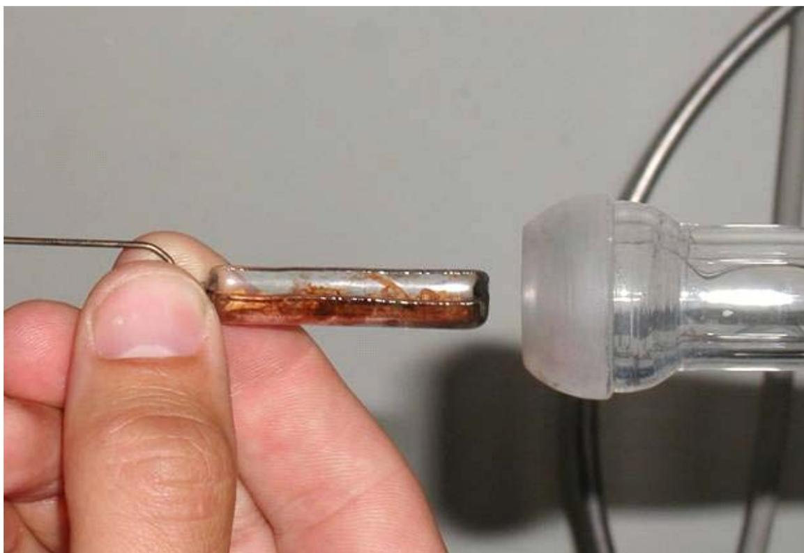
Figure 19: Photograph of the quartz boat containing a tobacco sample taken before being pushed into the quartz tube of the pyrolysis furnace
