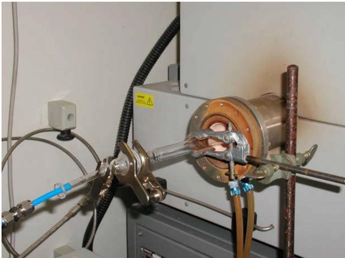
Figure 18: Inlet of the pyrolysis furnace and the quartz tube with the reaction gas line connected to the tube
