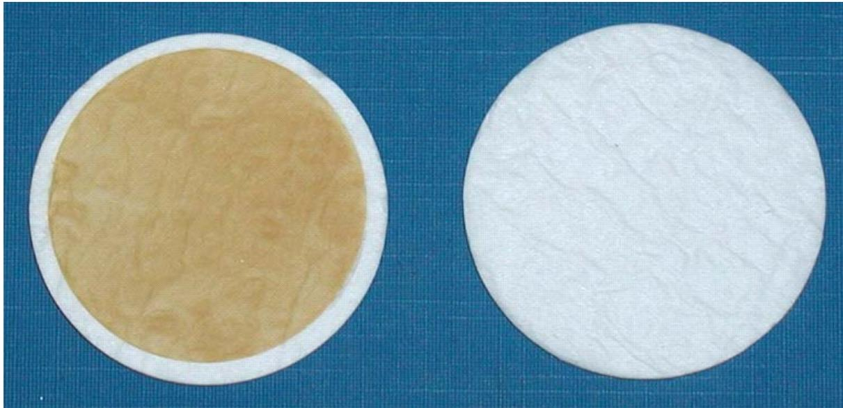
Figure 1: Photograph of a Cambridge filter pad (diameter 44 mm) before (right) and after (left) the smoking of one cigarette
