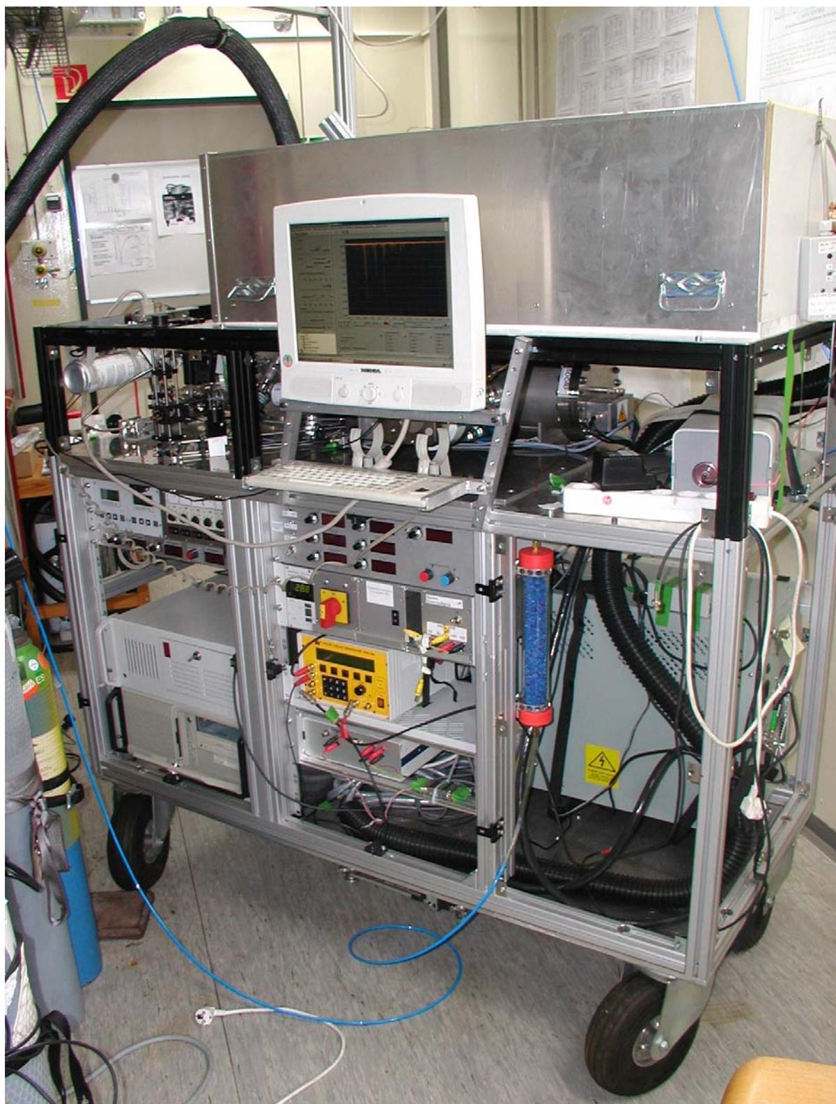
Figure 13 A: Photograph of the SPI/REMPI/EI-TOFMS instrument which was used for all the experiments in this work
