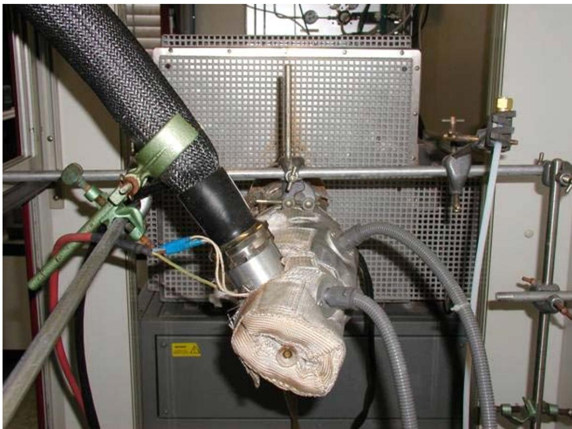
Figure 17: Outlet of the pyrolysis furnace with the quartz tube wrapped in heating mats and the transfer line of the SPI-TOFMS coupled orthogonally to the quartz tube
