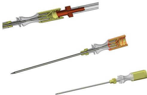
**Figure 3** Design of the coaxial positioning needle.
