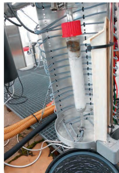
Fig. 7: The interior of the funnel adsorber sampler: in the upper part of the cartridge there is included glass wool in order to collect particulate matter, the white material in the lower part is the adsorbent (XAD-2 resin). Picture: GR, LfU
