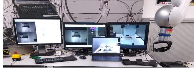
Fig. 7. Workplace for the human teleoperator. A LWR arm in mirrored joint configuration is used as haptic input device (top right section of the image). Different camera views (right screen: front view, middle screen: top view and visualization, laptop: side view) are available for the operator. The left screen displays the vision detection algorithm and is hidden during the user study.
