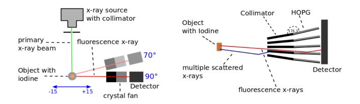
Figure 1: Left: Top view schematic of the x-ray fluorescence setup with analyzer crystal fan with 90° and 70° detector configuration; Right: Side view schematics of the HOPG crystal fan construction.
