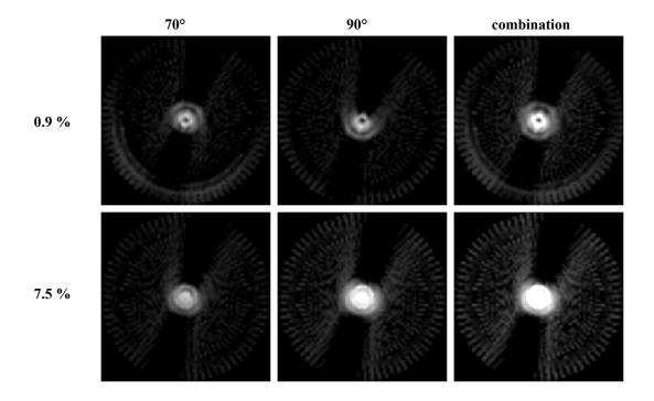
Figure 7: XFCT reconstruction images of the PMMA phantom for the detector configurations  $70^{\circ}$ ,  $90^{\circ}$ , and their combination, with iodine concentrations of 0.9 % and 7.5 %.
