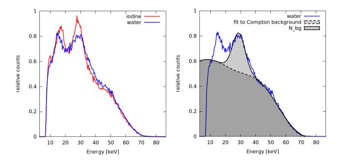
Figure 2: Left: Fluorescence measurements with a phantom containing simple water, also show an increased amount of photons with energies around that of the iodine  $K_{\alpha}$  fluorescence; Right: Approximation to the Compton background with a combination of quadratic functions. All spectra are normalized to the total number of counts.
