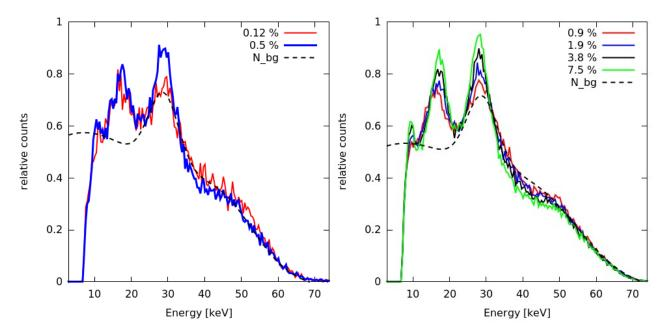
Figure 3: Recorded spectra of different iodine concentrations for the  $90^{\circ}$  detector configuration of the centric positioned simple phantom (l.h.s.) and the more complex phantom (r.h.s.), including a fit to the background. All spectra are normalized to the total number of counts.
