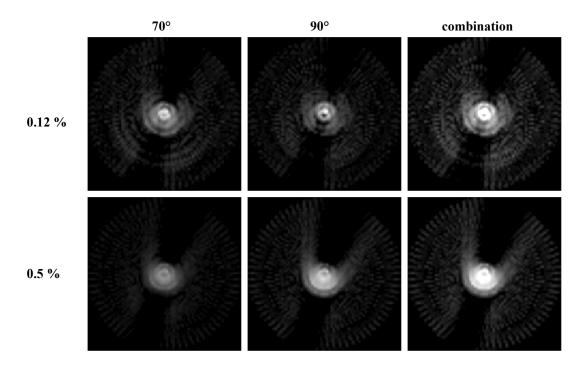
Figure 6: XFCT reconstruction images of the small phantom for the detector configurations  $70^{\circ}$ ,  $90^{\circ}$ , and their combination, with iodine concentrations of 0.12 % and 0.5 %.
