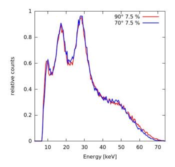
Figure 4: Comparison of the XRF spectra of the centric positioned large phantom containing an iodine concentration of 7.5 %, recorded in the conventional 90° detector-fan position and the 70° configuration. The spectra show no significant difference with regard to the distribution of the Compton photons.
