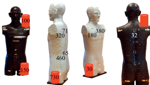
FIG. 5. Front and back view of setup 2 with reference dose rates (mGy).
