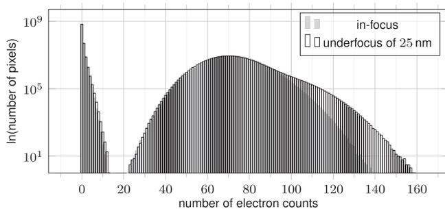
**Fig. 8. Effect of focus on dynamic range.** Distribution of electron counts for the full simulated 4D-STEM scan for 300 keV using an in-focus setting and an under-focus of 25 nm. The first peak of both distributions shows the dark field counts and the second, broader peak the bright field counts.
