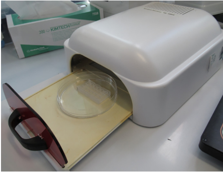
Figure 11. Chip placed in a 10 cm Petri dish in a custom-made UV sterilizer
