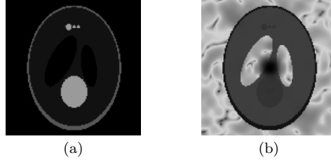
Fig. 2 (a) Background and (b) exemplary diffraction pattern perturbed by background noise in logarithmic scale.
