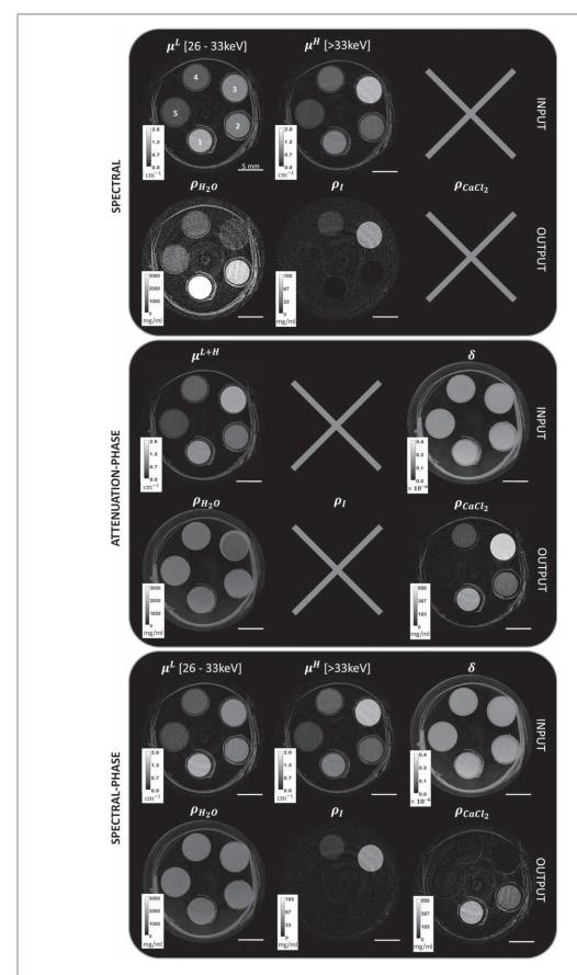
$\textbf{Figure 4.} \ Input tomographic reconstructions and material decomposition outputs of the cuvette sample for each tested algorithm, namely spectral, attenuation/phase and spectral/phase.\\$
