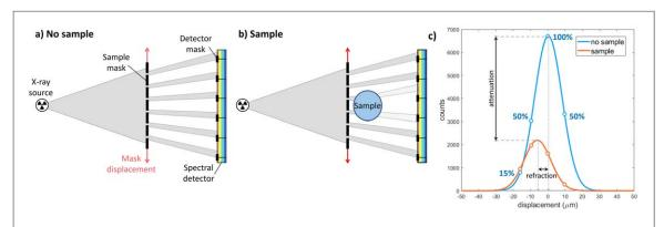
**Figure 2.** Sketch of an edge illumination setup without (a) and with (b) the sample. In (c), the illumination curves obtained without (blue line) and with (orange line) sample are shown. In the experiment, the curve was sampled the four points shown in the plots.
