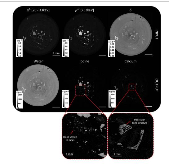
**Figure 5.** Input tomographic reconstructions and material decomposition output of the *post-mortem*  $\mu$ Angiofil®-perfused mouse sample using spectral/phase algorithm. In the third row, the zoomed-in details of the iodine and calcium maps.
