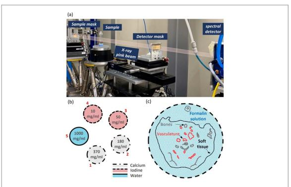
**Figure 3.** A photograph of the experimental setup (a) where the main components are outlined. In (b) and (c) the calibrated-cuvette sample and the mouse sample are sketched, respectively.
