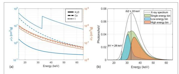
**Figure 1.** (a) Mass attenuation (blue) and phase (orange) coefficients as a function of energy of water, calcium, and iodine. (b) X-ray spectrum used for acquisition (dotted line) and energy spectral response of the system (area-filled curves).
