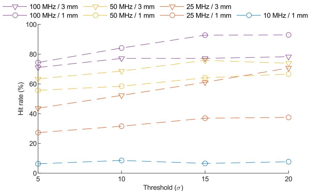
**Figure S2: Hit rate in respect to the camera signal threshold for all pIDTs measuring beads.** The camera threshold is given in multiples of the standard deviation of noise ( $\sigma$ ). An increase of the threshold results overall in an increase of the hit rate, but reduction in the number of detected particles.
