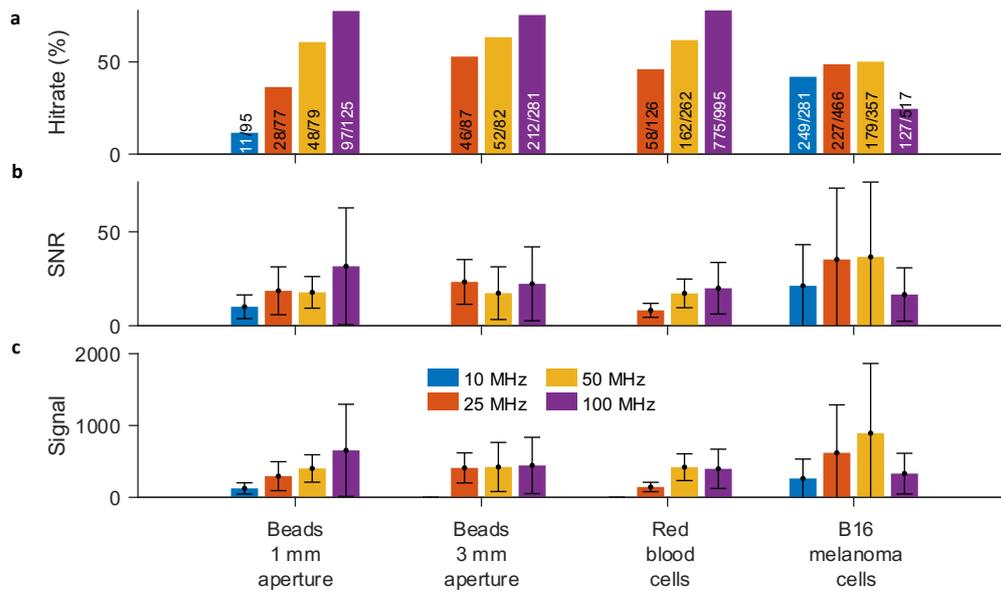
**Figure S6: Characteristics of the measurements regarding OA signal, SNR and hit rate.** In the (b) and (c) bars depict the mean, the error bars depict the standard deviation. Due to the dimension of the pIDT, there is no 10 MHz chip with a 3 mm focal length. Red blood cells could not be detected using the 10 MHz pIDT.
