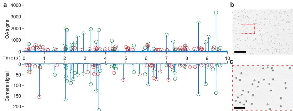
**Figure S5: Exemplary traces of 3  $\mu\text{m}$  polystyrene beads.** (a) Trace of 3  $\mu\text{m}$  beads. This measurement was done using the 100 MHz pIDT with 3 mm focal length. 48 events were co-registered out of 65 events detected by the camera (74% hit rate). (b) Microscope image of an aliquot of 3  $\mu\text{m}$  beads (scale bar 125  $\mu\text{m}$ ). (c) Section of (b) (scale bar 25  $\mu\text{m}$ ).
