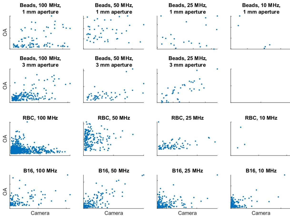
**Figure S7: Correlation of camera and OA signal for co-registered events.** First row shows beads measurements with the 1 mm focal length pDTs, second row beads measurements with the 3 mm focal length pDTs, third row red blood cells, fourth row B16 cells. Each column shows the measurements of a single pDT (100, 50, 25, 10 MHz).
