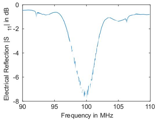
**Figure S4: Frequency characteristics of electrical reflection coefficient  $|S_{11}|$ .** Shown is exemplary the coefficient for an 100MHz pIDT with 1mm focal length
