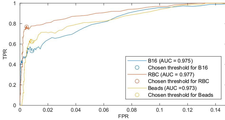
**Figure S3:** Receiver operating characteristic (ROC) curves exemplarily shown for measurements using the 50 MHz pIDT with 3 mm focal length. The chosen threshold of  $5\sigma$  shows a good balance between high true positive rate (TPR), while keeping the false positive rate (FPR) to a minimum.
