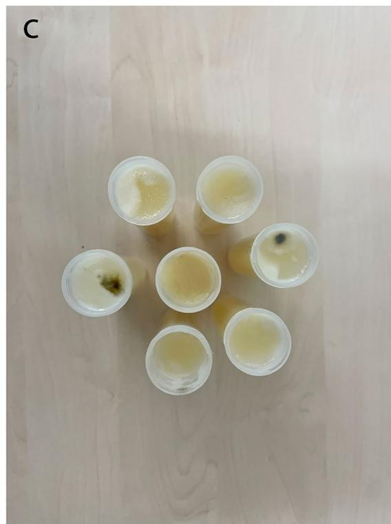
weeks. **b** Comparison of T2 times measured at baseline and after 4 weeks. **c** Photograph of the test phantoms (batch 1) after a storage period of 4 weeks—mold growth is clearly visible on some phantoms
