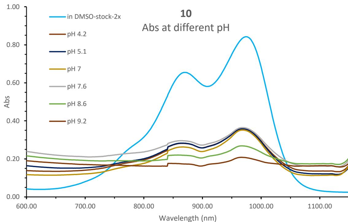
**Figure S8.** Absorption spectra of **10** at different pH ranges (DMSO stock Conc. 50  $\mu$ M, and 20  $\mu$ M prepared by diluting the DMSO stock solution with aqueous buffer in 5:2 ratio)
