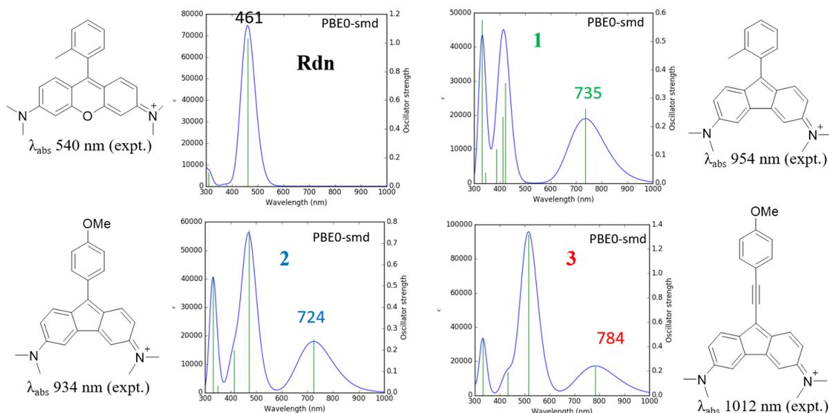
**Figure S13a.** The TD-DFT (PBE0, in water) predicted optical spectra with oscillator strength (y-axis) of three dyes (**1-3**), along with rhodamine (Rdn) for comparison to estimate the prediction error.
