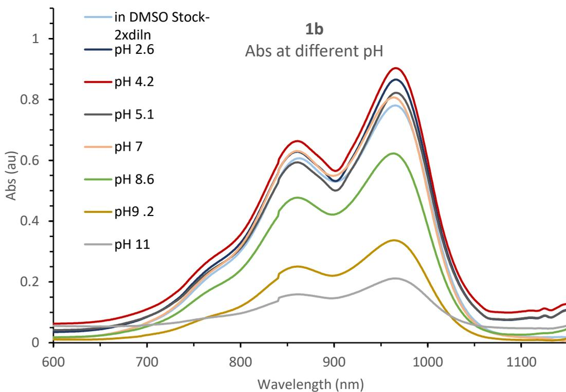
**Figure S7.** Absorption spectra of **1b** at different pH ranges (Conc. 50 $\mu\text{M}$ , prepared by diluting the DMSO stock solution with aqueous buffer in 1:1 ratio)
