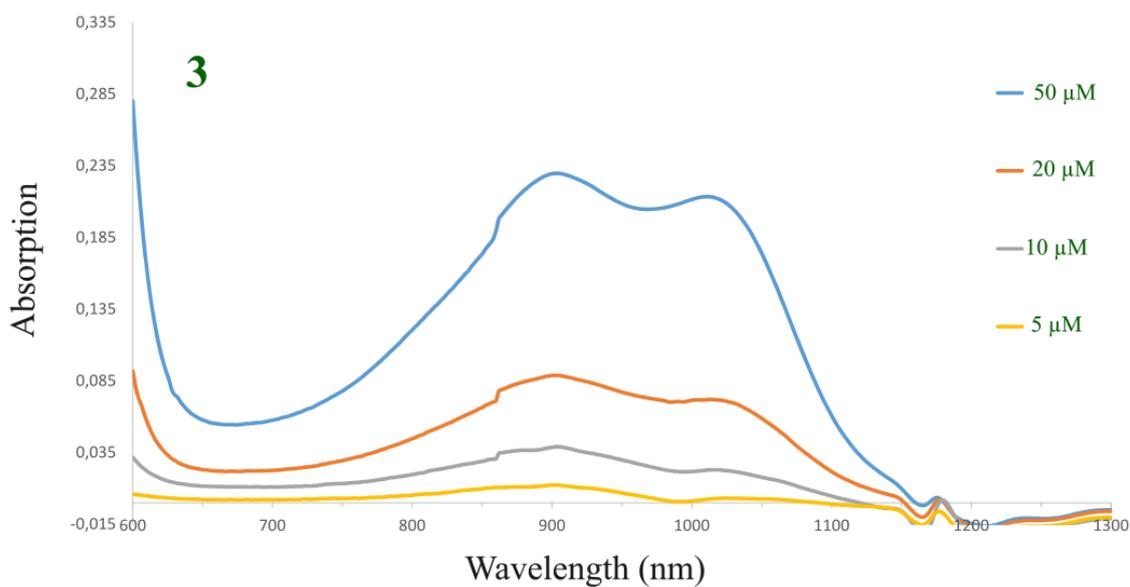
**Figure S6.** Absorption spectra of **3** at concentrations ranging from 50  $\mu\text{M}$  (blue), 20  $\mu\text{M}$  (orange), 10  $\mu\text{M}$  (grey) and 5  $\mu\text{M}$  yellow
