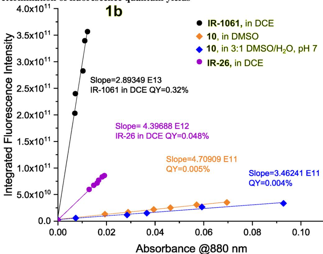
**Figure S11.** Determination quantum yield ( $\Phi_f$ ) of **1b** with respect to IR-26 and IR-1061 as reference, based on integrated fluorescence intensity vs absorbance (previously determined  $\Phi_f$  of IR-26 = 0.048%, and IR-1061 = 0.32% in DCE).
