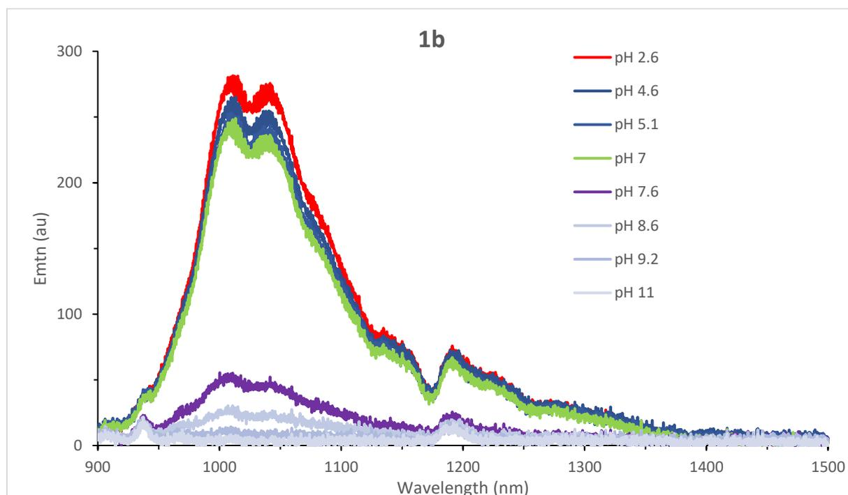
**Figure S9.** pH dependent fluorescence emission spectra of **1b** (with a 880 nm long pass filter, conc. 25  $\mu$ M); quenching in basic buffer medium was observed.
