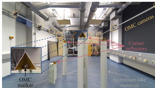
FIGURE 4. A photograph of the measurement setup shows corner reflectors with optical motion capture (OMC) markers attached positioned in front of the radar to align the coordinate systems. The OMC cameras, highlighted by yellow circles, track the markers' positions. For accurate registration of the radar and OMC coordinate systems, a common target must be detectable at the same location by both systems.
