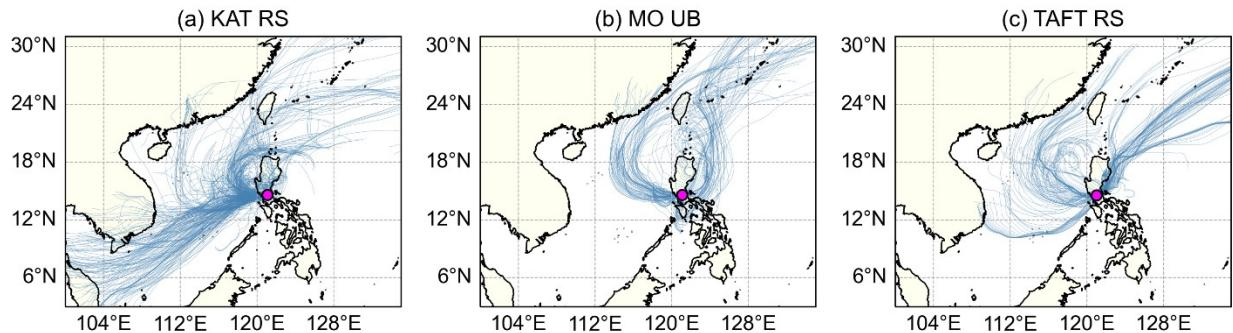
**Figure S2:** HYSPLIT back trajectories for (a) KAT RS, (b) MO UB and (c) TAFT RS, with those locations denoted by the pink circles in each respective panel. Results shown are based on five-day back trajectories generated every hour using GDAS data at 500 m above ground level.
