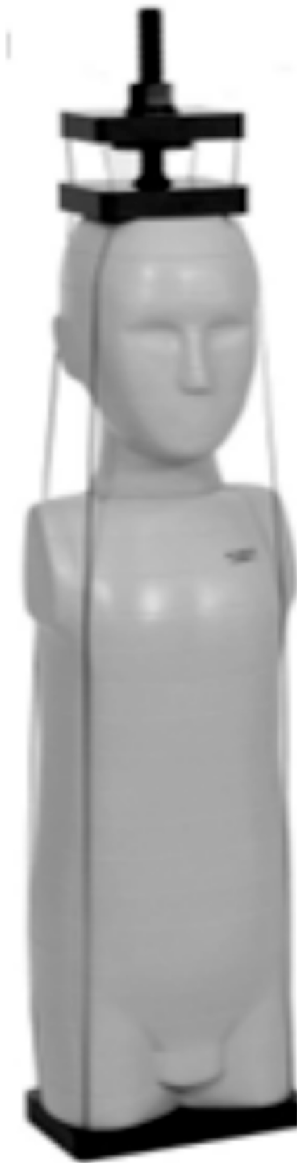
Fig. 3. Anthropomorphic phantom CIRS ATOM 705 (ABEL) [12].
