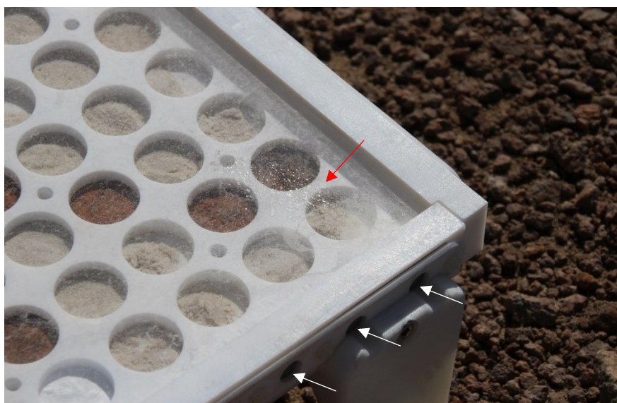
Figure S 1 Dew formation (red arrow) in the sample plates below the glass cover on the 31st of January 2023. Air vents (white arrows) are located on the side of the plate.
