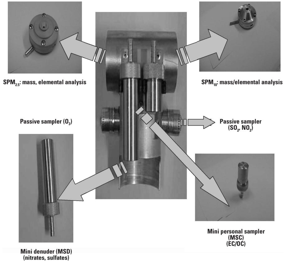
**Figure 12.** Diagram of the multipollutant personal sampler (Demokritou et al. 2001). Abbreviations: EC, elemental carbon; MSC, mini personal sampler; MSD, mini denuder; OC, organic carbon; SPM, suspended particulate matter.
