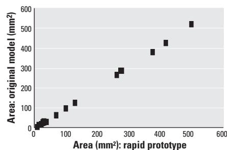
**Figure 7.** Cross-sectional luminal airway surface of original hollow airway cast made from a normal human tracheobronchial tree in square millimeters versus corresponding airway surface in square millimeters of a replica produced by STL using data obtained by CT scanning of the original cast.
