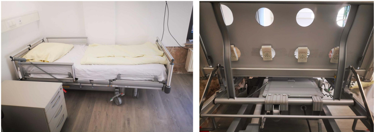
Fig. 2. Study setup for radar-based sleep monitoring. (Left) The clinical sleep laboratory environment with a hospital bed used for overnight recordings. (Right) The underside of the bed frame, showing the placement of the radar sensors.
