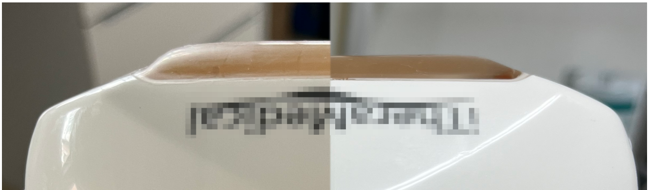
Figure S2. Membrane filling inconsistencies cause positional offsets between devices. In a manufacturer-provided example using two additional MSOT Acuity Echo probes, incomplete or uneven membrane transducer filling was associated with an approximately 3 mm positional shift of the membrane position relative to the imaging plane. For comparison, the in vivo dataset in Fig. S1 showed a smaller between-device skin-depth offset of approximately 1.6 mm. This observation suggests that membrane filling differences are a plausible contributor to the positional offsets observed in the in vivo dataset between devices 1 and 2 and can potentially be further amplified by operator-dependent pressure differences. Beyond inconsistent filling procedures, membrane properties are susceptible to temporal changes such as scratches or contamination, which can generate further systematic image artifacts 1 . Photo courtesy of Braden Eliason (iThera Medical GmbH).
