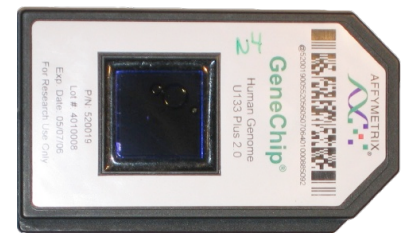
Figure 2.3: An Affymetrix® GeneChip® Retrieved March 10, 2010, from http://www.wikipedia.com
