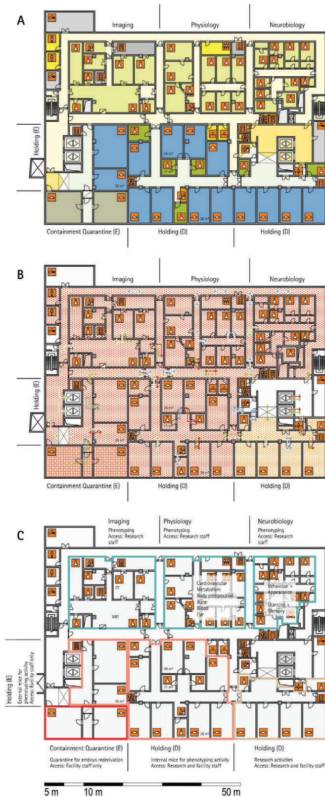
Figure 2. Schematic floor plans—facility 1, plan 2. (A) Zoning scheme. (B) Flow and hygiene levels scheme. (C) Functional unit scheme. For a description of the icons and colors used in the floor plans, see the legend to Figure 1.
