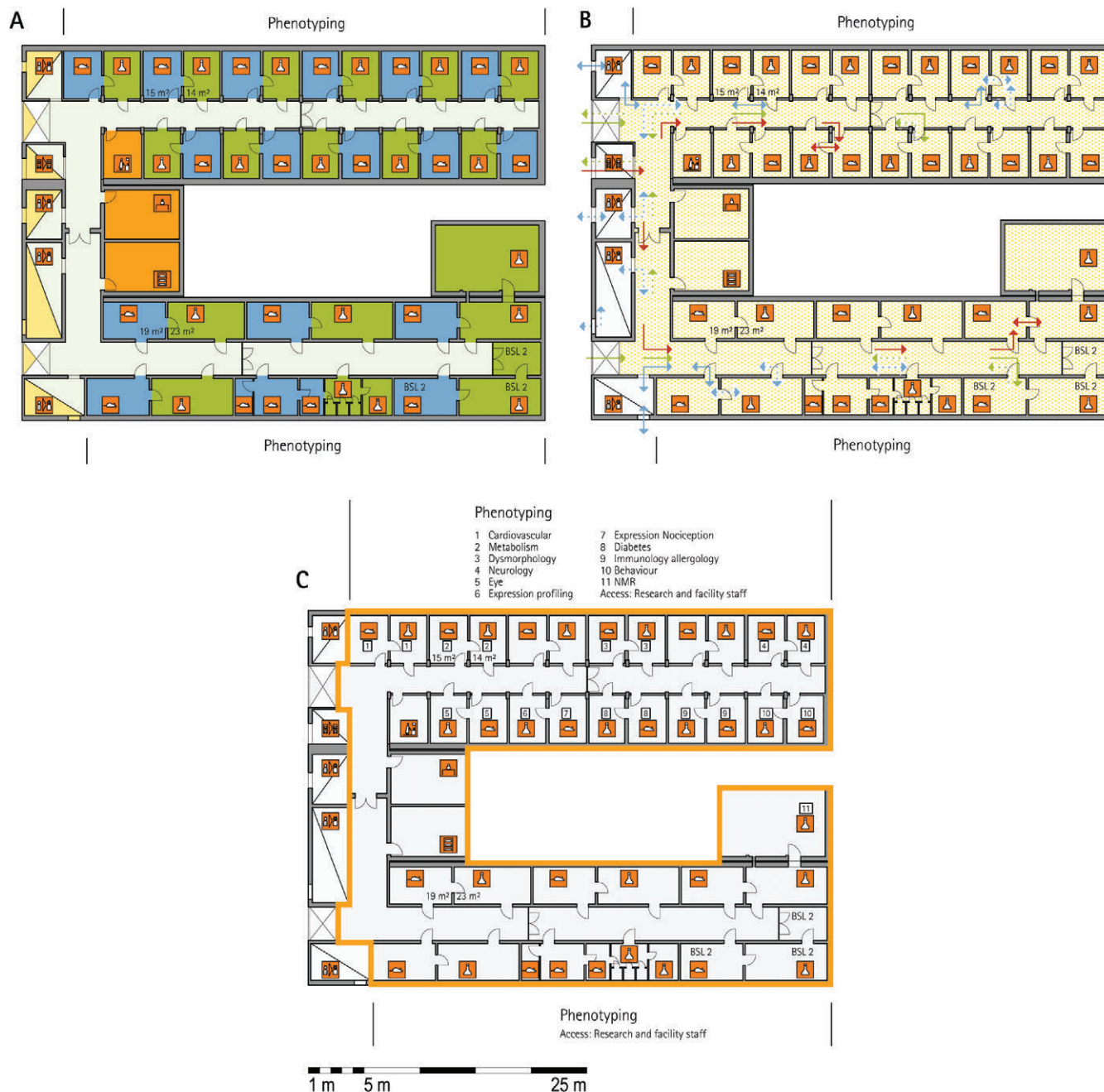
Figure 5. Schematic floor plans—facility 2, plan1. (A) Zoning scheme. (B) Flow and hygiene levels scheme. (C) Functional unit scheme. For a description of the icons and colors used in the floor plans, see the legend to Figure 1.
