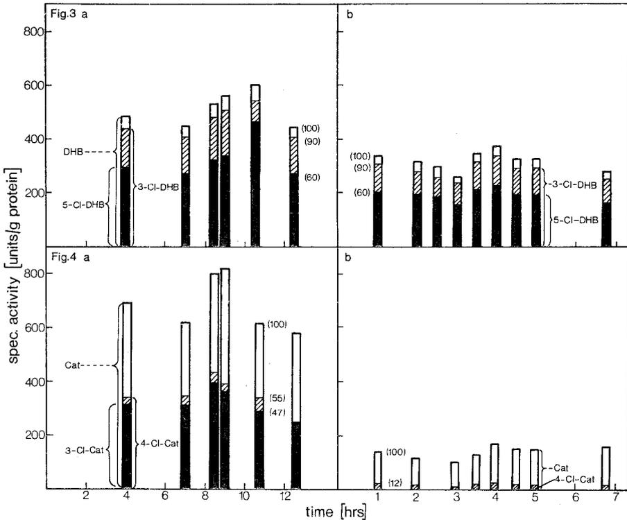
Fig. 3a and b. Specific activities of DHB dehydrogenase in cell free extracts from cells harvested at certain intervals during growth in a fermenter (see Fig. 1) on 3-chlorobenzoate (a) and benzoate (b). (—) 3,5-cyclohexadiene-1,2-diol-1-carboxylic acid (DHB) and its 3- and 5-chloro-analogues (3-Cl-DHB and 5-Cl-DHB) were added as substrate. The numbers in parentheses give the relative activities for the different substrates ( $DHB = 100$ )
