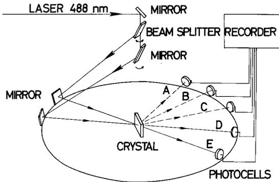
**Fig. 13.** Experimental set up (schematic) for associative volume coupling. Rotatable beam splitter and mirrors generate two coherent laser beams interfering with arbitrary angles at the place of the central crystal. Writing starts with wave *A* and *B*, then the orientation of wave *A* is changed in order to generate wave *C*. The second hologram is taken with waves *B* and *C*. Then wave *B* is rotated to become wave *D* and the waves *C* and *D* form another hologram etc.
