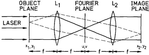
Fig. 1. 4- $f$ -arrangement, an optical image processing set up. The lens system  $L_1, L_2$  images the object plane onto the image plane. The image is inverted with respect to the object orientation. Parallel coherent illumination (expanded laser beam) generates the spatial frequency spectrum (Fourier transform) of the object in the back focal plane of lens  $L_1$
