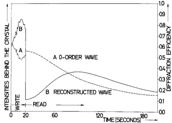
**Fig. 10.** Associative storage and reconstruction of two plane waves. The storage period is 20 s, showing an interaction of the nascent diffraction index pattern and the generating interference pattern (wave *B* gains energy of wave *A*). After 20 s wave *B* is blocked and reconstruction takes place with the energy of wave *A*. Wave *B* shows selfenhancement due to energy loss of the recalling wave *A*. After some time both waves decay because of an increasing scattering of the crystal
