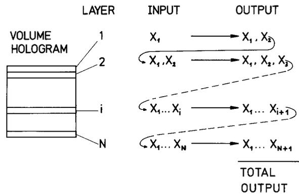
**Fig. 11.** Schematic volume coupling. All holograms  $H_1 = |X_1 + X_2|^2$  ...  $H_N = |X_N + X_{N+1}|^2$  are incoherently superposed on the tridimensional storage material. Each layer is a complete multiply exposed hologram. Any arbitrary input element recalls its next neighbour out of any arbitrary layer. The just recalled elements will recall the following neighbours out of the following layers, thus reconstructing the complete associative chain step by step
