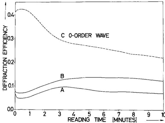
Fig. 14. Associative chain of three elements. *O*-order wave *C* reconstructs the neighbored wave *B* and the cross-coupled wave *A*. Both recalled waves *B* and *A* show selfenhancement
