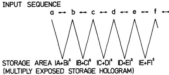
Fig. 4. Associative chain. The input patterns are time-sequentially presented in pairs. Each pair is stored holographically, forming the holograms  $H_1 = |A+B|^2$ ,  $H_2 = |B+C|^2$  and so on. Holograms  $H_1 \dots H_N$  are superposed one above the other, yielding a multiply exposed hologram
