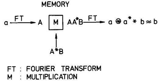
Fig. 2. Reconstruction scheme. Pattern  $a$  initiates the reconstruction of pattern  $b$ . Input pattern  $a$  is Fourier transformed ( $A$ ) and multiplied by the transparency of the holographic memory. The product of the incoming pattern and the stored pattern gives  $AA^*B$  and after another Fourier transform the pattern  $b$  approximately
