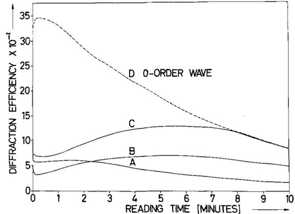
Fig. 15. Associative chain of four elements, *O*-order wave *D* reconstructs the waves *C*, *B*, and *A* with changing diffraction efficiency. Note that the two-fold cross-coupled wave *A* comes out more strongly than the previous wave *B* within the first two min of reconstruction
