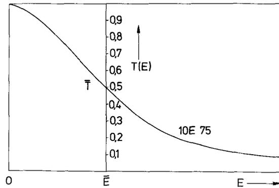
**Fig. 7.** Amplitude transmission of Agfa Scientia 10 E 75 plates (after Goldman, 1976),  $E$  exposure,  $T(E)$  amplitude transmission
