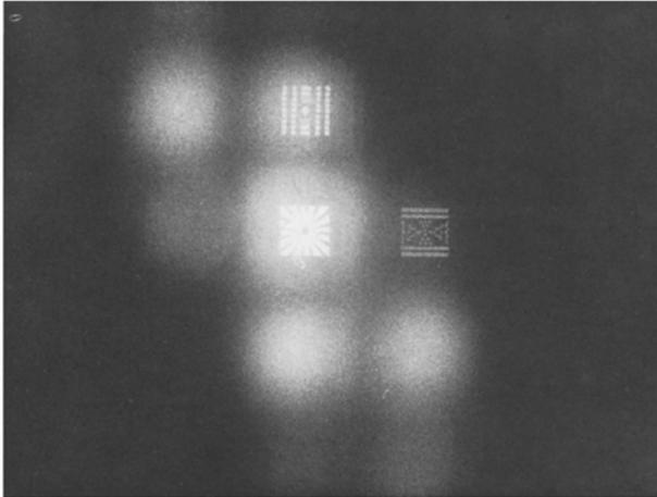
**Fig. 8.** Nonlinear coupling. The star-like pattern (centre) is linearly coupled to the pattern of rectangular dots (top) and by quadratic nonlinearities to the striped and dotted pattern (right). The star-like pattern reconstructs both patterns although the striped and dotted pattern (right) didn't exist simultaneously with respect to the centre pattern. The bright stains are disturbing cross-correlation terms
