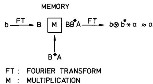
Fig. 3. Reconstruction scheme. Pattern  $b$  initiates the reconstruction of pattern  $a$ . Input pattern  $b$  is Fourier transformed ( $B$ ) and multiplied by the transparency of the holographic memory. The product of the incoming pattern and the stored pattern gives  $BB^*A$  and after another Fourier transform the pattern  $a$  approximately
