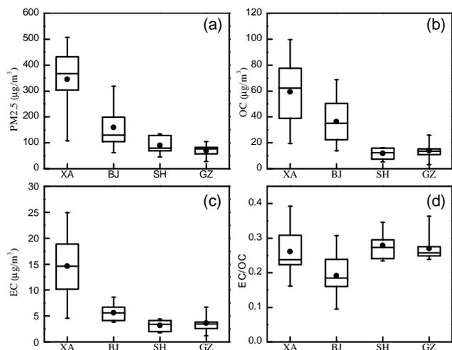
**Figure 1.** Box-and-whisker plots of mass concentrations of  $\text{PM}_{2.5}$  (a), OC (b) and EC (c) and EC/OC ratios (d) for samples collected in Xi'an (XA), Beijing (BJ), Shanghai (SH) and Guangzhou (GZ) during the winter of 2013. The box represents the 25th (lower line), 50th (middle line) and 75th (top line) percentiles; the solid dots within the box represent the mean values; the end of the vertical bars represents the 10th (below the box) and 90th (above the box) percentiles.
