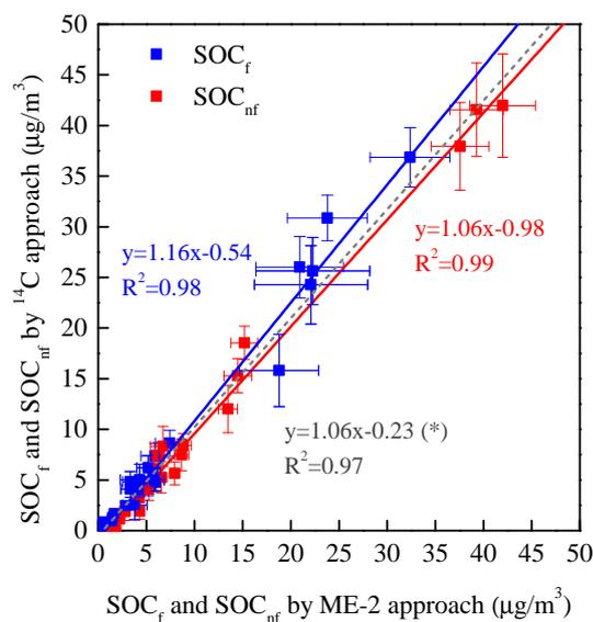
**Figure 7.** Comparison of secondary OC from fossil and non-fossil sources (i.e.,  $\text{SOC}_f$  and  $\text{SOC}_{nf}$ , respectively) resolved by the  $^{14}\text{C}$  and ME-2 approaches. The dashed line denotes a linear regression fit of  $\text{SOC}_f$  when excluding data from Beijing, yielding an alternative regression slope marked with an asterisk (\*). Note that the intercepts are insignificant for all three cases.
