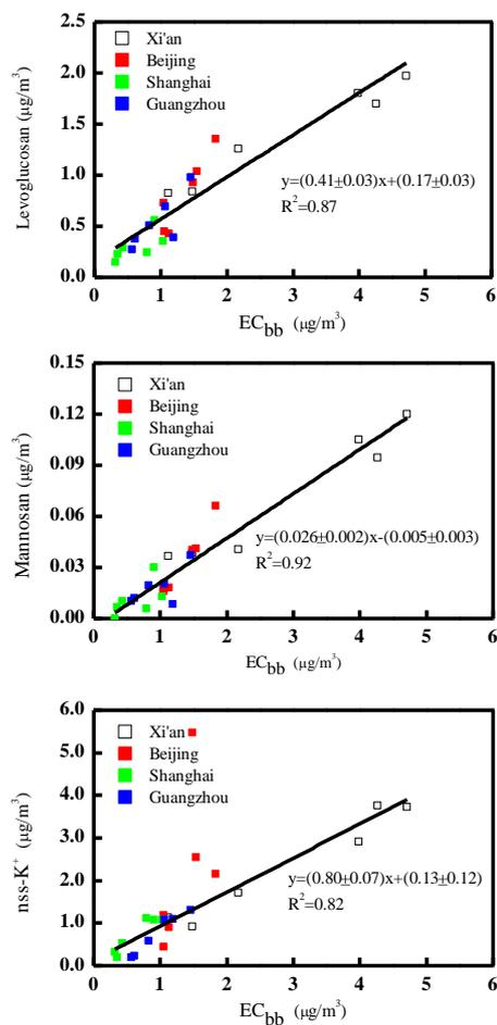
**Figure 4.** Scatter plots of concentrations of  $\text{EC}_{\text{bb}}$  with levoglucosan (top), mannosan (middle) and non-sea-salt potassium (nss-K<sup>+</sup>, bottom).
