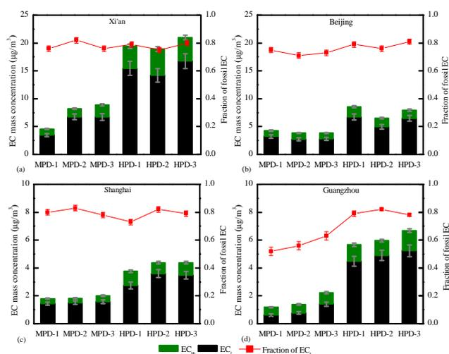
**Figure 2.** Mass concentrations ( $\mu\text{g m}^{-3}$ ) of EC from biomass burning and fossil-fuel combustion ( $\text{EC}_{\text{bb}}$  and  $\text{EC}_f$ , respectively) as well as fractions of fossil EC to total EC for aerosols samples in Xi'an, Beijing, Shanghai and Guangzhou during moderately polluted days (MPD) and heavily polluted days (HPD). Note the different scaling for the northern and the southern cities.
